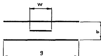
Fig. 1. Strip transmission line.
